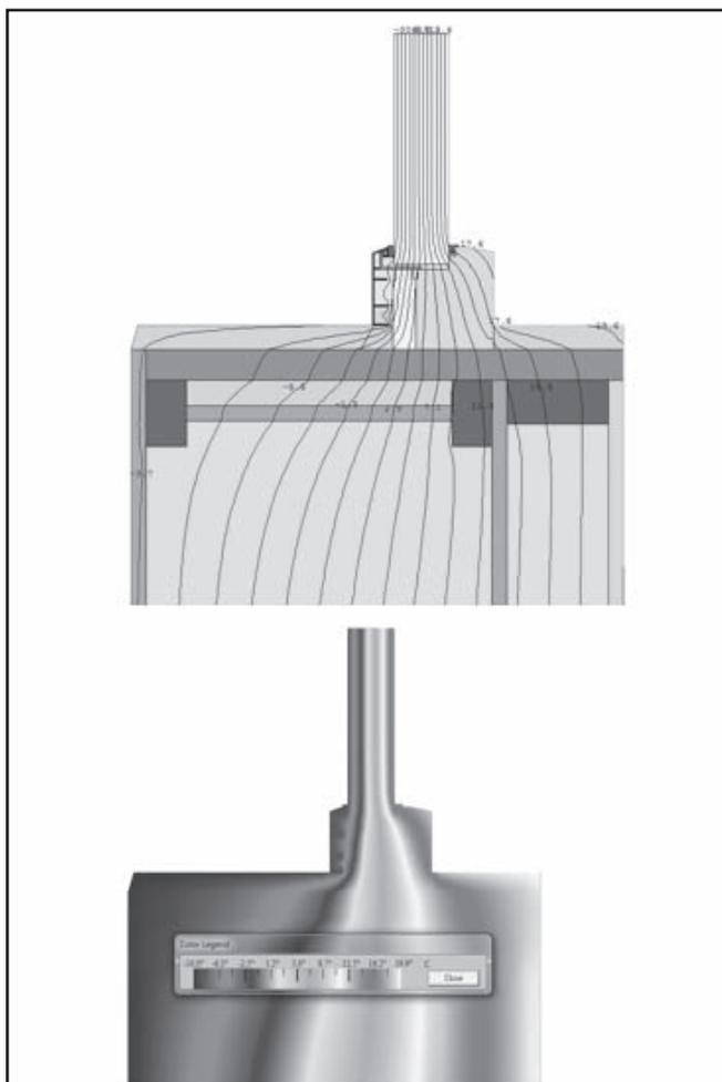
Figure 9. If we add ½” of over-insulation inside and outside, the PSI install becomes negative: -0.005 BTU/hr\*ft²\*F. The overall wall is now performing better than the simple sum of wall and window. Image courtesy Zola Windows.
