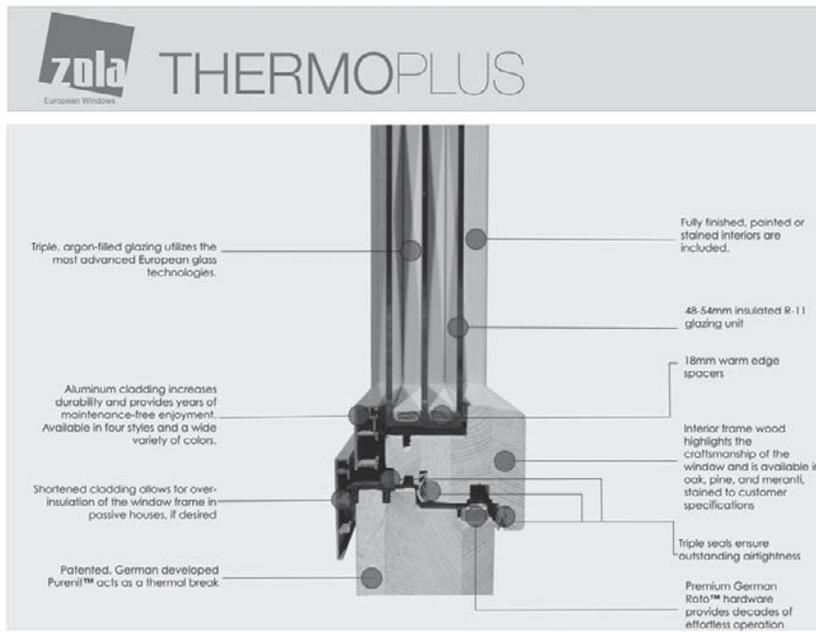
Figure 6. Detailed cutaway of a Zola Window. Figure courtesy Zola Windows.
