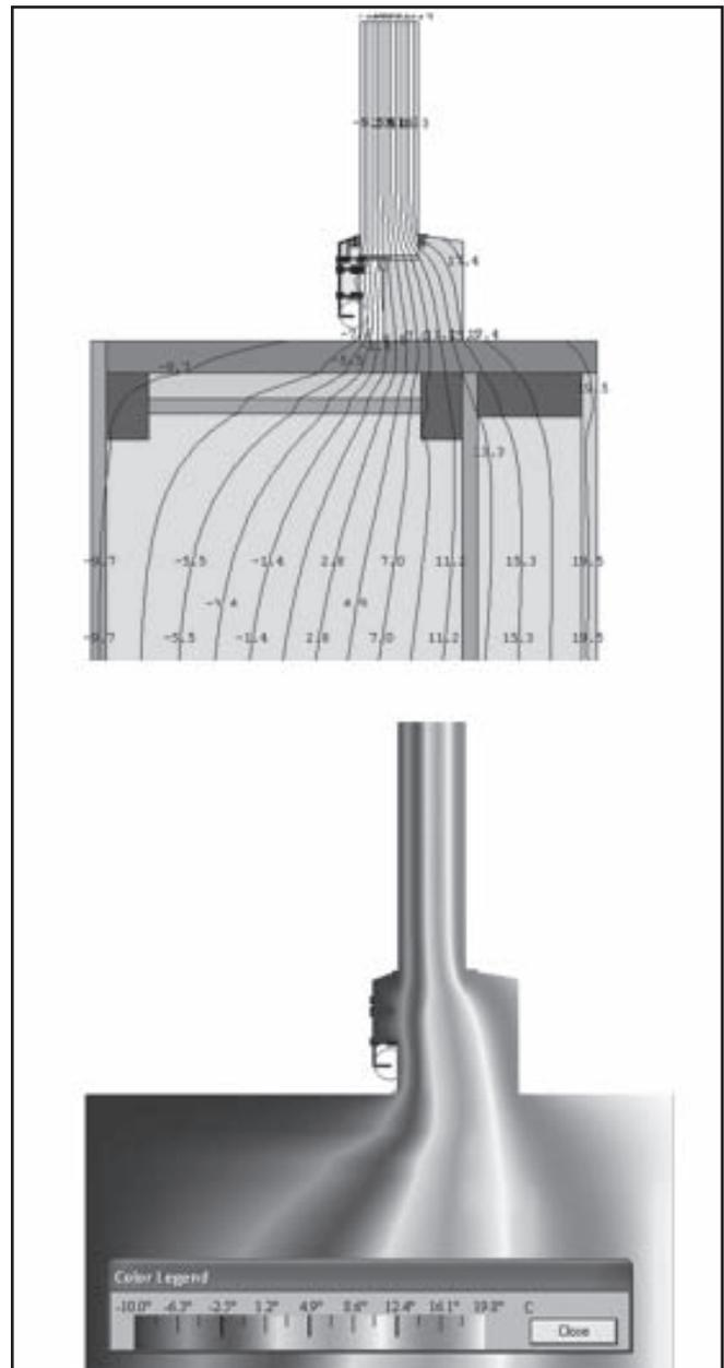
Figure 8. The same wall assembly and window, but with the window centered over the insulation. The PSI install drops to 0.014 BTU/hr\* $ft^2$ \*F as calculated by THERM. Image courtesy Zola Windows.
