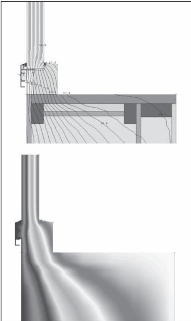
Figure 7. Outside flush install. The Psi install is calculated at 0.023 BTU/hr\* $ft^2$ \*F. Image courtesy Zola Windows.
